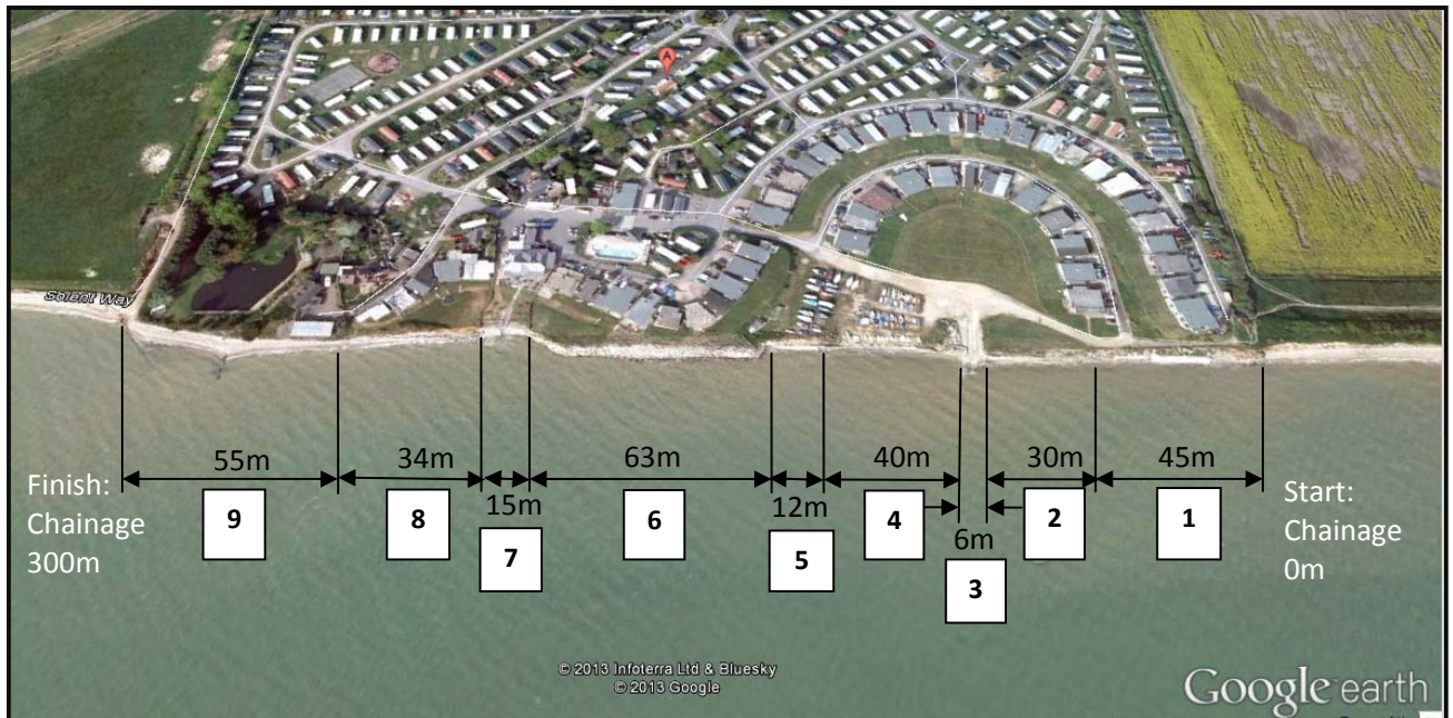
Figure 2: Solent Breezes defence lengths identified during the site visit (image copyright: Google Earth)
